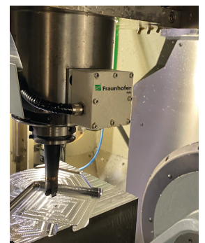
Our sensorbox with acceleration sensor attached to the milling spindle for condition monitoring
